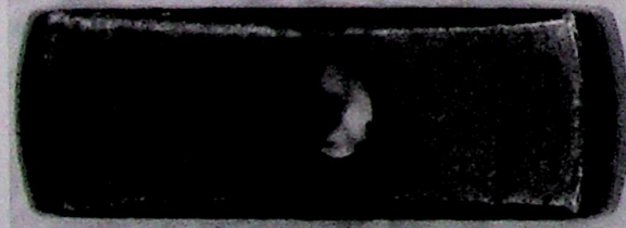
Type I lock bar, smaller hole 6-40 NF thread. Observed on rifles 500,000 March 1942 to 1,100,00 December 1942.
