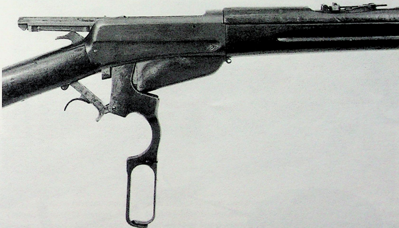
Fig. 3 – Close up of the open action with lever down of US marked Winchester Model 1895, S/N 17893. Photo Tim Prince, College Hill Arsenal.
