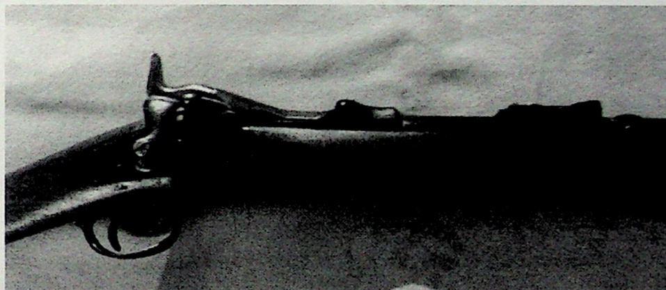
Right: 1873 Cadet right side with coarse checkered hammer, 1873 rear sight, and cadet trigger guard
