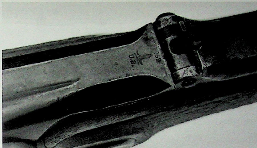
ABOVE: 1869 Breech Block of carbine. It is dated 1869, stamped with American Eagle and U.S. All parts are similar to 1869 rifle. The receiver is the longer type made before the model 1870.
