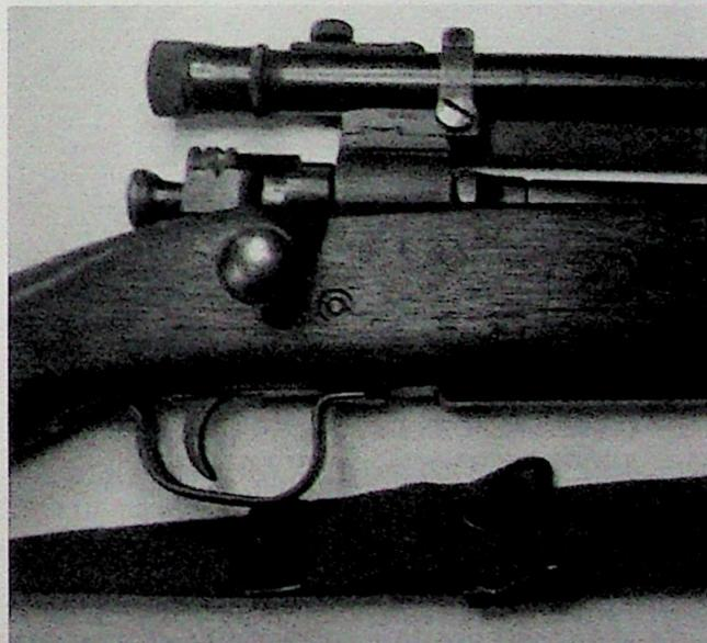
1903A4 Showing Lowered Bolt Cut and Receiver modification for the low bolt.
