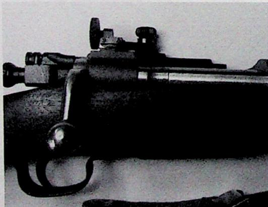
Redfield Olympic receiver sight mounted on the left side of the receiver with 5 adjustment positions. Standard 1903A3 rear sight was removed. Other 1903A3 fittings were normally used.
