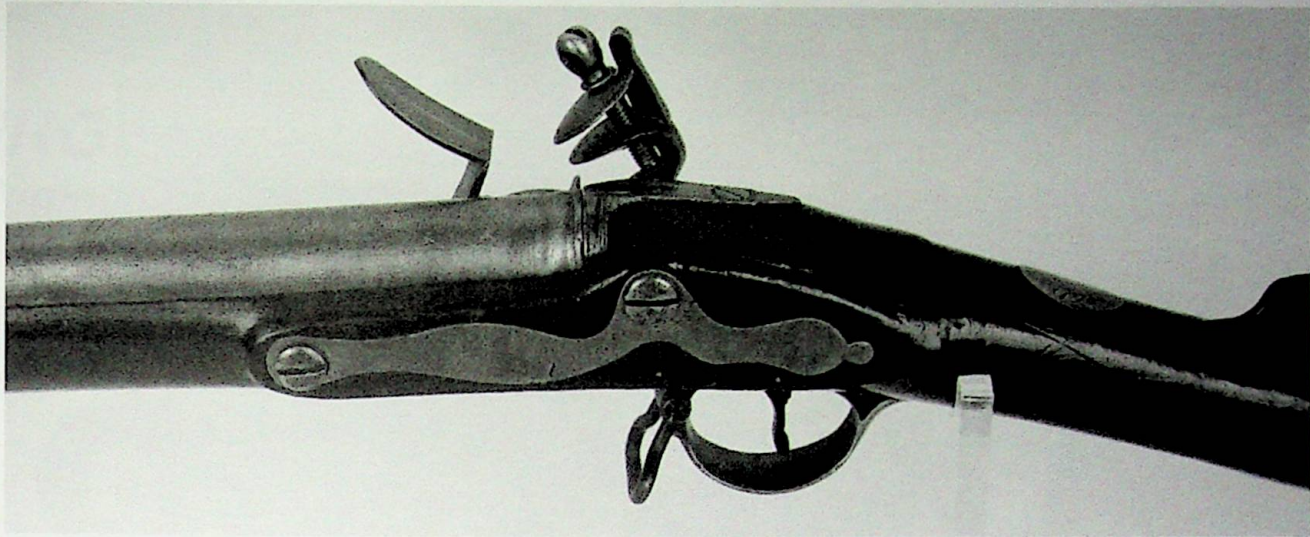
Above: Right side showing two screw side plate, trigger guard swivel, and stock.
