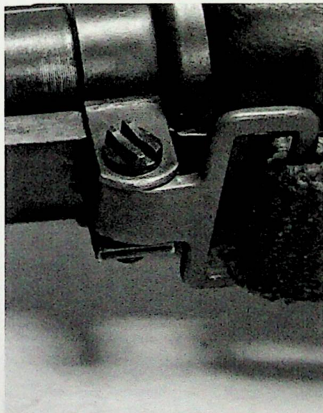
Above: Sling Swivel with Machined Screw Cloth Sling, Crisp machining and stamping and machine marks on barrel. No bayonet fixture.
