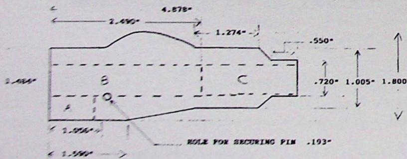
addition of a steel "blob" to the muzzle. The 5-in. long muzzle attachment, which is solid except for having a polished bore for the bullet to pass through, is secured by a cross pin; the barrel has been cut to 26" in length and turned down for 2.5" at the muzzle with a notch made on the bottom to accommodate the cross pin. The muzzle of the barrel is also counterbored to a depth of
